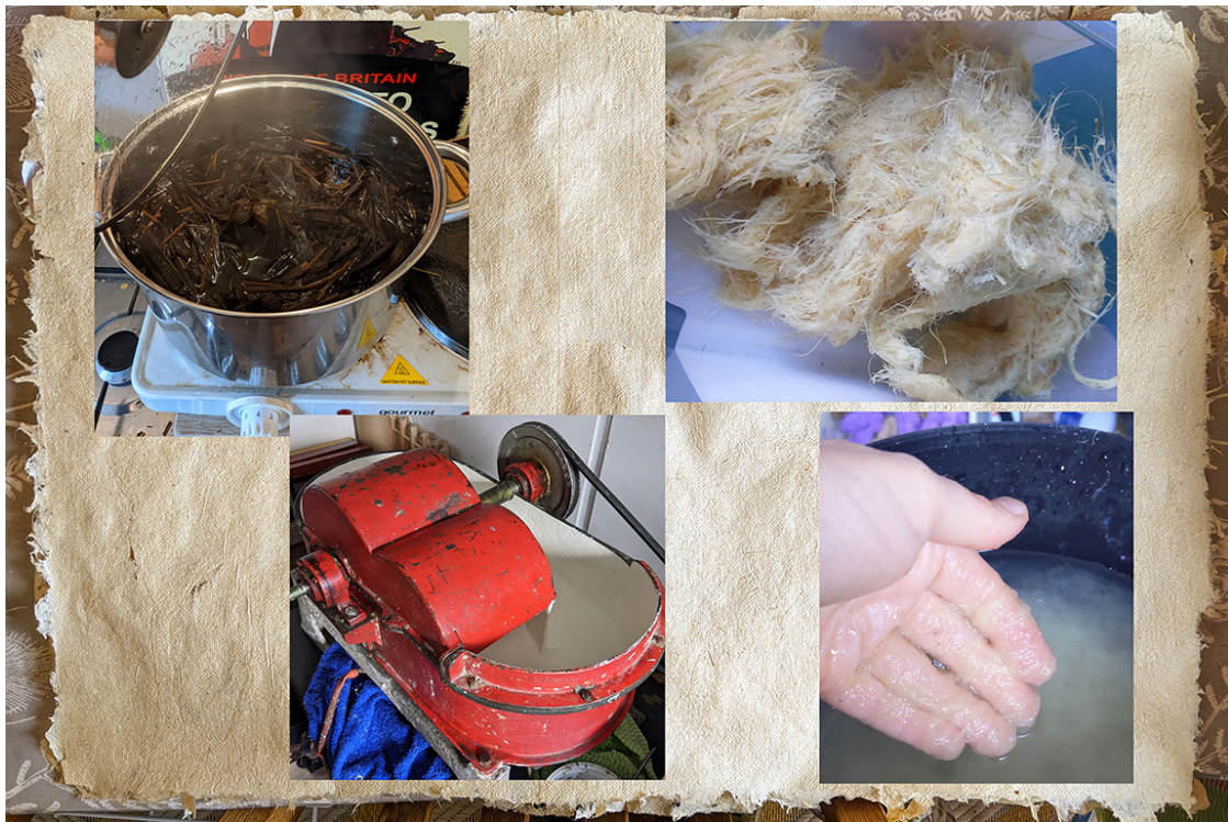
Image 5: Graffiti carvings, selection of test pieces made from plaster, paper, lino and moulding silicone Image 6: Cooking plant fibres, bleached fibres, Hollander beater, and beaten fibres suspended in water
